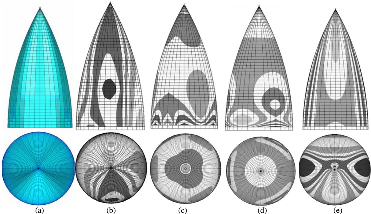
Figure 1: Ogive surface normal displacements for grinding forces and Twyman stress
