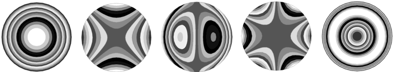
Figure 4.2 Applied Zernike Surface Displacements from left to right; focus, astigmatism, coma, trefoil, and spherical aberration.
