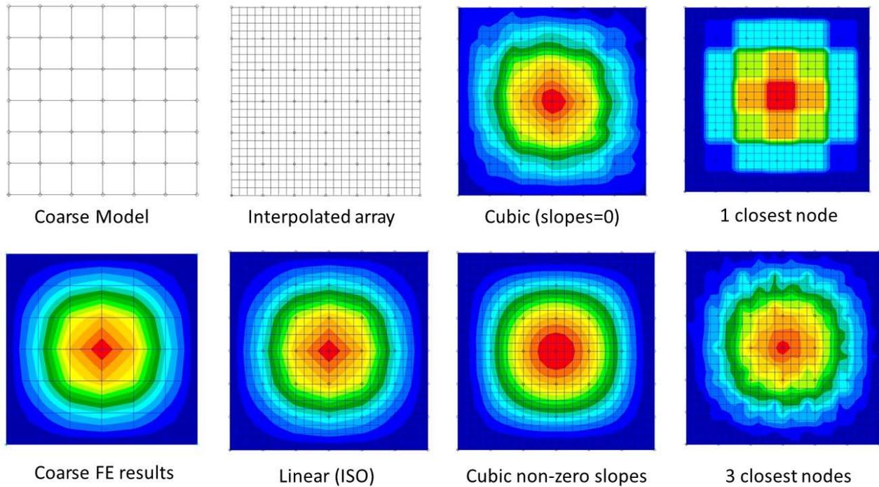
**Figure 3: Comparison of interpolation techniques**
