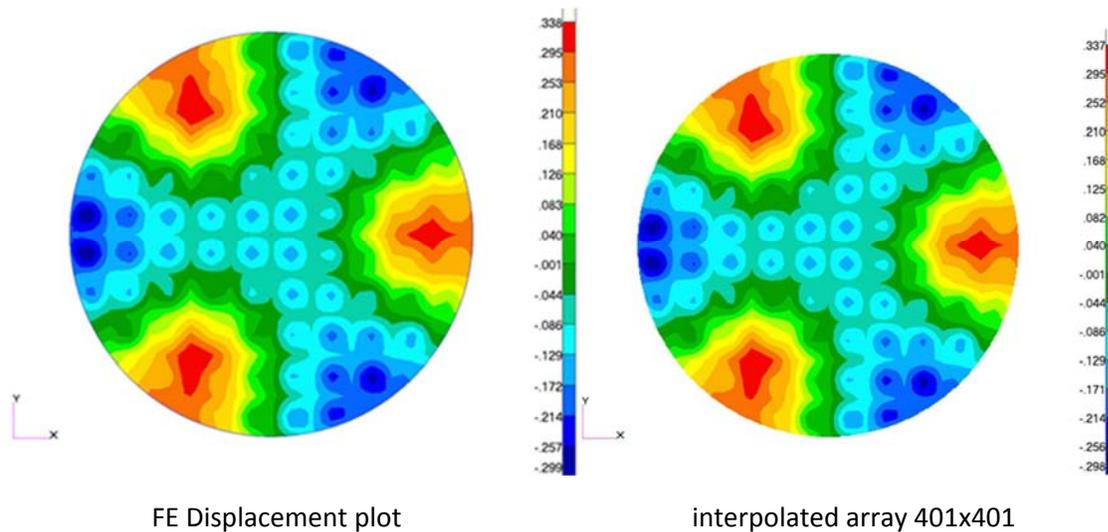
**Figure 2: Interpolation on a light weight mirror with quilting**
