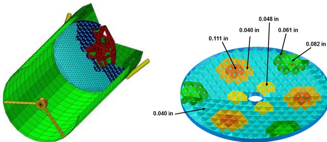
**Figure 12: Telescope and optimized adaptive primary mirror**
