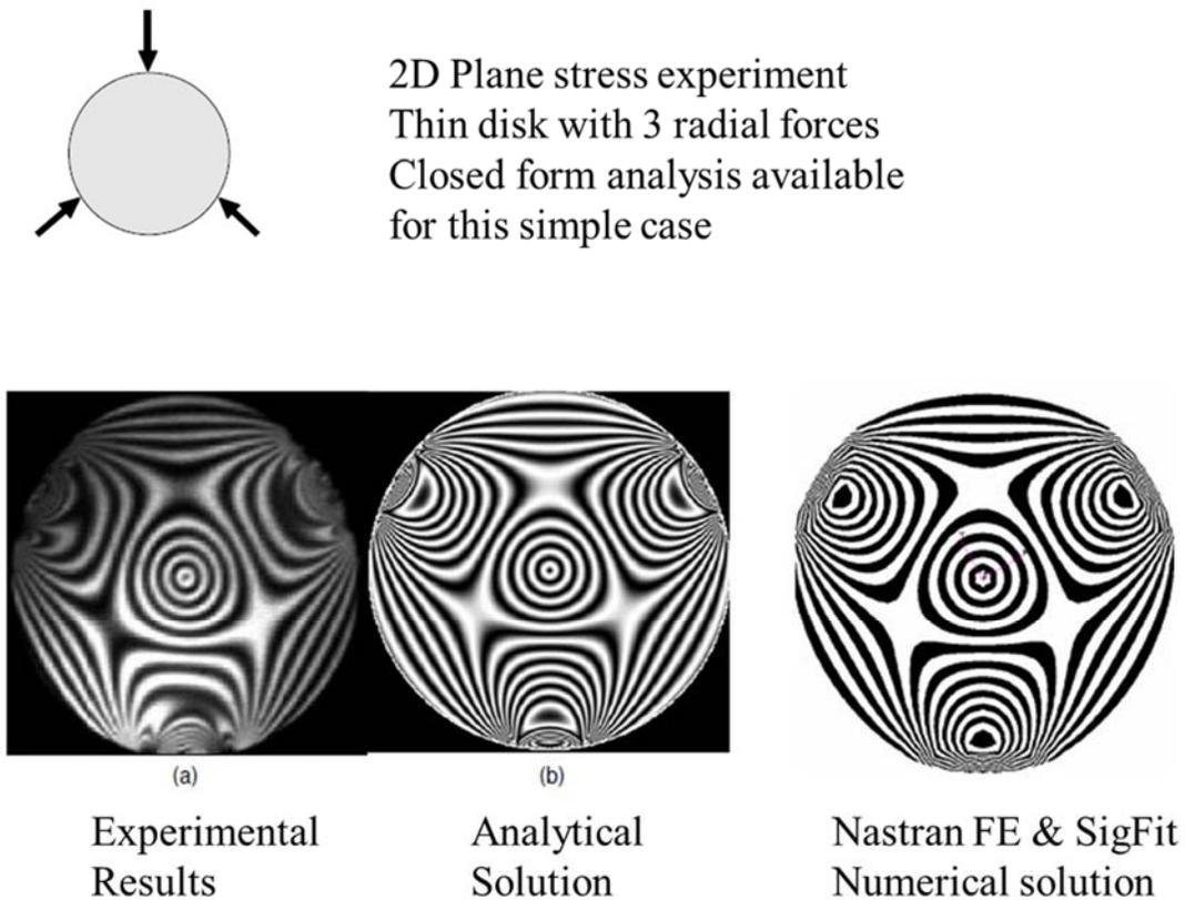
Figure 10: Comparison of birefringence from test and analysis
