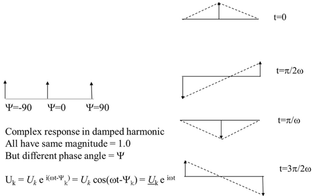
**Figure 5: Harmonic response with equal magnitudes but different phases**
