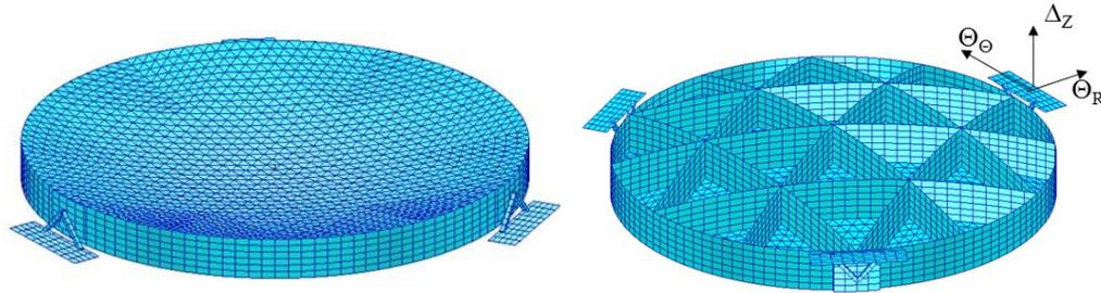
**Figure 11. Mount flatness and coplanarity**
