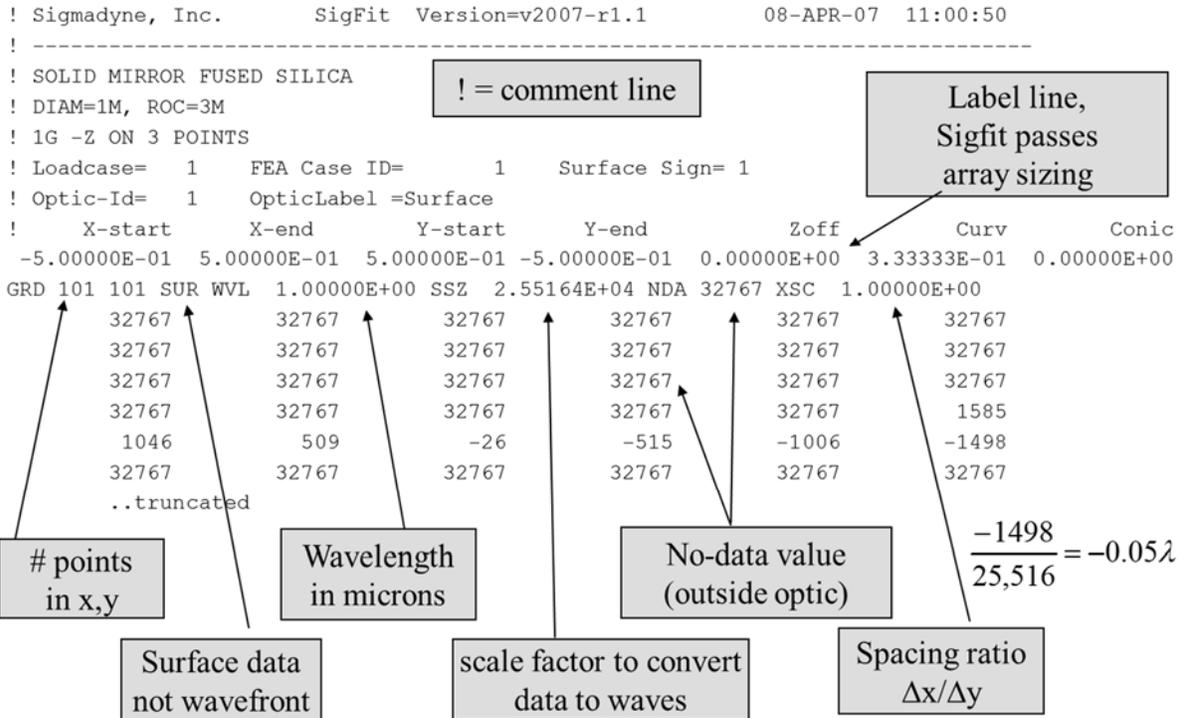
**Figure 4: interferogram grid array file**
